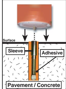
L - Clean area of any stones, gravel or solidified resin, remove plastic cap with flat head screw driver, insert T-Bar into top of post and screw into the pre-installed sleeve.
