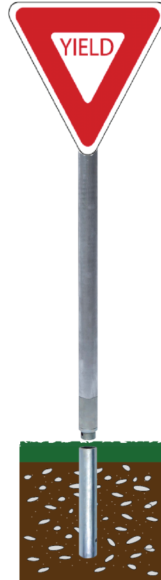
Ground Sleeve Earth or Concrete foundation
